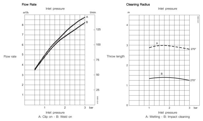
**Note:** The inlet pressure has been taken immediately before the inlet to the machine. In order to achieve the performance indicated on the curves, the pressure drop in the supply lines between pump and machine must be taken in consideration and the water temperature during testing was approx. 20°C.
